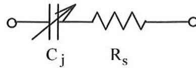
Fig.7-2 The equivalent circuit of varactor diode
